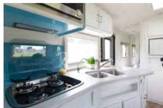
The Villa's ergonomically-designed kitchen area is conveniently laid out and well equipped with a three-burner Thetford Spinflo gas powered cooktop complete with its own recessed glass lid. You also get a full size microwave and beautiful stainless steel double sink with a separate tap for filtered drinking water, an extended mixer tap and included sink covers.
