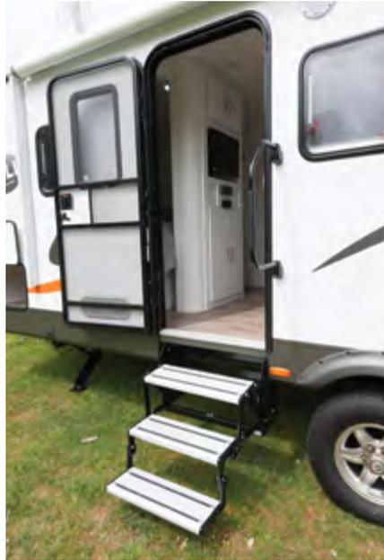
Even with its elevated ground clearance, getting in and out of your Villa is easy thanks to a couple of intelligent design elements. The door itself has been built extra-wide for greater accessibility with two-way fly-screen entry. A folding, three step ladder from Tread Lite opens down easily to give you reliable footing all the way up.
