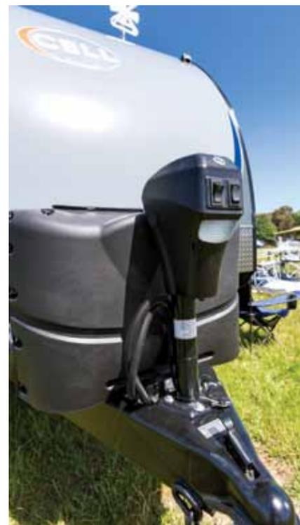
Forget worrying about the winding, with a 12V front power jack that allows you to lift the caravan on and off your car with zero effort. You will be relieved to know that it is no longer a scary experience winding on and off in the dark, with a handy built-in night light. The winch also contains a manual override button in case of power loss. Also mounted on the A-frame are two 9kg gas bottles, safely encased in a hard plastic covering.
