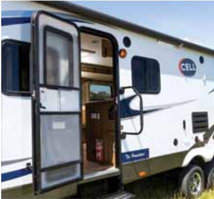
To ensure your van can combat Australia's tough climate without hesitation, the Homestead is constructed from Alumi-X welded aluminium that sits under an outer layer of Lamilux 4000 fibreglass walls. The foam brick insulation in the walls and roofing, as well as insulation batts in the floor, give you the perfect climate-controlled home from which to explore this amazing country.
